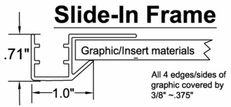
Slide-In frame can accept maximum of 1/4"~.250" as max thickness.
