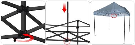
The frame will have one canopy tensioner at the center of the underside. Carefully turn the handle counter-clockwise to eliminate tension on the canopy. This will lower the canopy and simplify disassembly.
