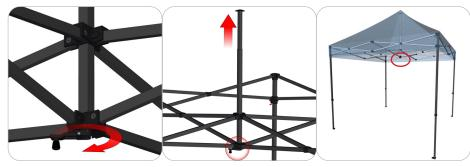
The frame will have one canopy tensioner at the center of the underside. Carefully turn the lever clockwise to create tension on the canopy. This will raise the canopy and eliminate wrinkles.
