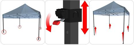
The frame will have four slide locks, one for each corner. When the tent scissor frame is fully extended; make sure the prong of the slide lock snaps into the tube locater hole. Press the lever on the slide lock to disengage the prong from the tube allowing to slide the lock up or down during assembly.
