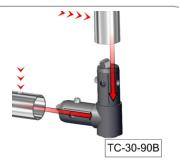
Use TC-30-90B for bottom corners. Connect sides of frame to elbow joint by pressing snap buttons.
