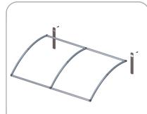
Once frame is connected attach feet. It is best to assemble with frame still laying flat. See next step for detail.
