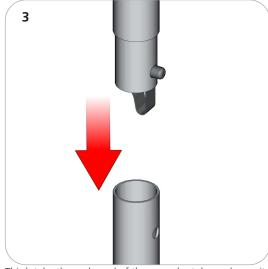
Third, take the male end of the spreader tube and snap it in place of the back wall snap button connectors.
