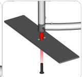
Take the plastic connector and make sure the snap buttons are in proper position for the frame tube holes. Simply press the snap button with your thumb and carefully slide the tube onto the connector. The snap button should pop through. Some twisting may be necessary to assure the snap button has popped all the way through the tube hole. Do not force the connection and be careful with the tube edges, they may be sharp.
