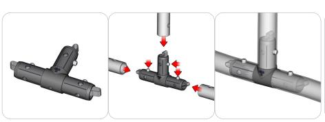
Take the plastic connector and make sure the snap buttons are in proper position for the frame tube holes. Simply press the snap button with your thumb and carefully slide the tube onto the connector. edges, they may be sharp.
