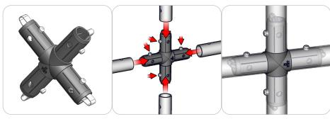
Take the plastic connector and make sure the snap buttons are in proper position for the frame tube holes. Simply press the snap button with your thumb and carefully slide the tube onto the connector. The snap button should pop through. Some twisting may be necessary to assure the snap button has popped all the way through the tube hole. Do not force the connection and be careful with the tube edges, they may be sharp.
