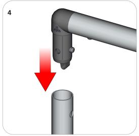
Fourth, take the male end of the plastic connector and snap it into the spreader tube open end.
