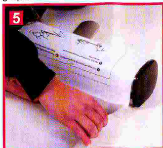
5 Attach the bottom of the graphic banner to the leader strip. Back of graphic attaches to the tape.
